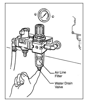
Figure 4-5 – Air Line Filter
